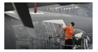
An Australian aviation startup has developed an adhesive film inspired by shark skin that reduces drag on aircraft due to its sandpaper-like texture.
